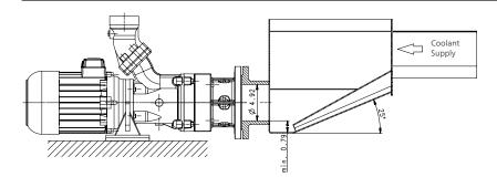
SBC pumps are comparable to SFC pumps from a technical standpoint. When directly mounted to the tank or to the machine tool preventive actions must be taken in order to avoid unwanted foreign objects, such as broken tooling pieces, from reaching the pump suction.
