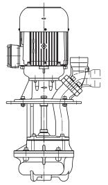
Vortex pumps are traditional lift pumps with a recessed impeller that allows for a sphere passage of up 50 mm. In order to ensure stable operating conditions the impeller must be fully flooded, and the pump must lift the fluid at least 10–25 inch (3–8 m) above the pump discharge.
