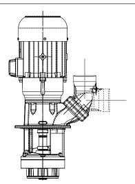
The cutter pumps of the series SPC are designed to handle and reliably cut long, stringy plastic chips.
