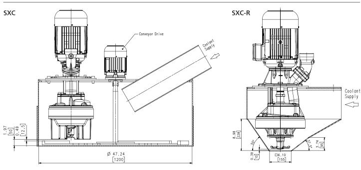
The cutter pumps of the series SXC are designed to handle low alloyed steels, machining steel (SXC-H) and cast iron / aluminum combinations (SXC). Chips can also be in the shape of birds nests or chip bundles.
