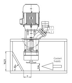
The cutter pumps of the series SFC are suited for cutting aluminum chips or similar materials and for pumping these materials along with the coolant fluid. An agitator located at the pump suction helps to break up and separate any large bundles of chips or birds nests which reach the pump suction.
